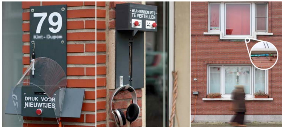
Figure 2. StreetTalk , consisting of three situated public displays that allowed messages to be printed ( Readl , left), audio fragments to be listened to ( Listen , middle), and ambient sound levels to be visualized ( Shush , right).
